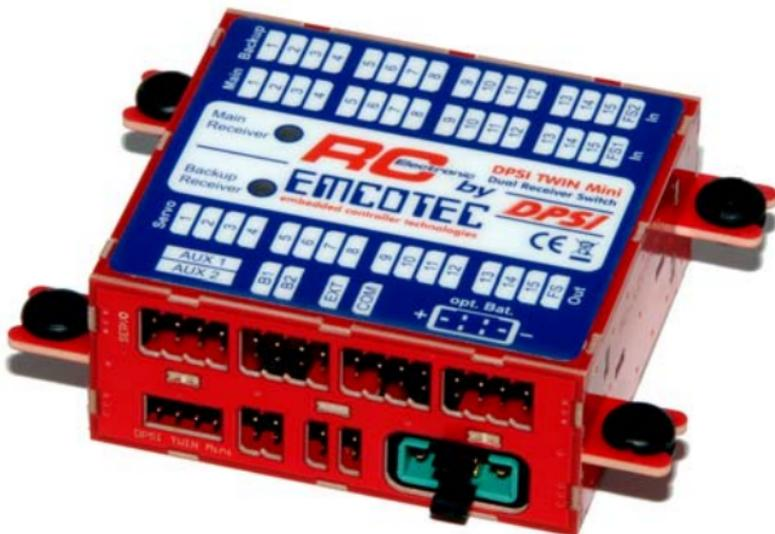
You find the pin connectors of the outputs in the upper row (connections to servo current distribution or to the servos directly).
