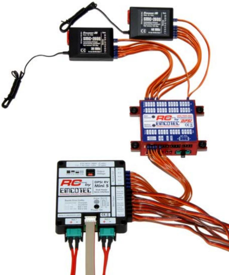
In this example, the DPSI RV Mini is used as a current distributor. The **DPSI TWIN Mini** serves just as receiver switch and is supplied with voltage by the DPSI RV Mini 5 via the patch cables. Both receivers are supplied from the **DPSI TWIN Mini** via their patch cables.
